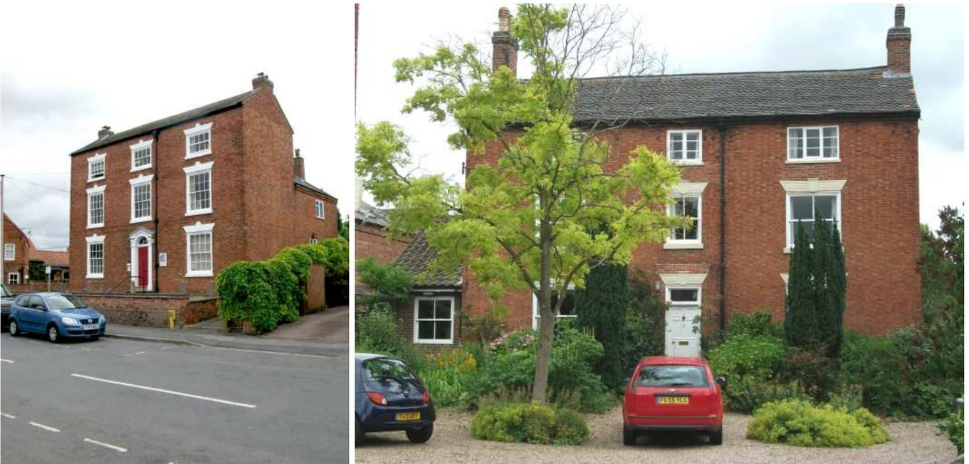
Above left: 19 Main Street is an eighteenth century house built in the Georgian style with well set red brick walls, slate roof and a regular pattern of sash windows placed symmetrically around a central doorway with fanlight. Above right: 17 Main Street is a substantial early nineteenth century yeoman's house with a distinctive machine tile roof, red brick gable stack and symmetrical frontage.
