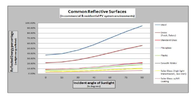
It should be noted that the reflected energy percentage of Solar Glass is far below that of a standard glass and more on the level of smooth water. Also, below are the ratios of the common reflective surfaces:
