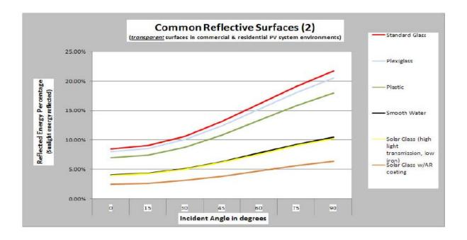
Light beam physics resolves that the least amount of light is reflected when the beam is the normal, in other words, least light energy is reflected when the beam is at 0 degrees to the normal. The chart below is a result of light beam physics calculations:
