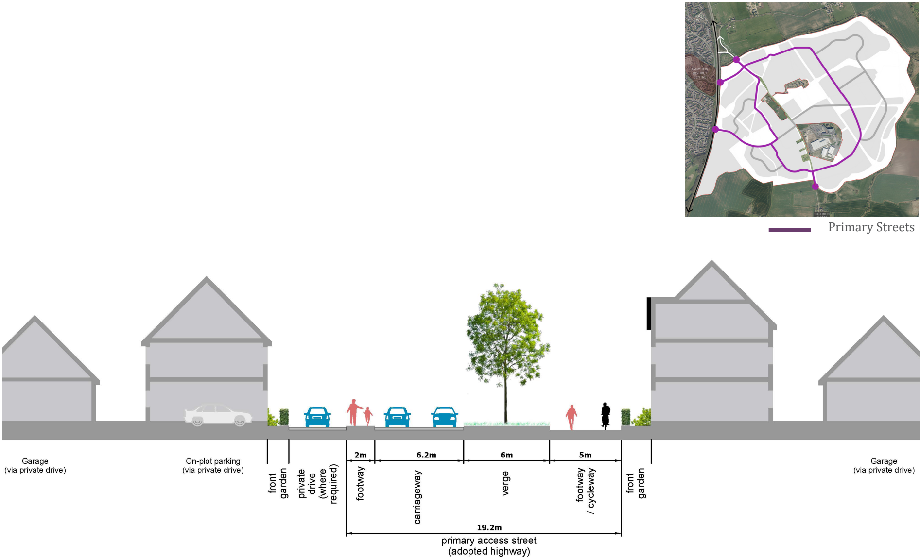
Figure 36. Indicative Primary Street Section
